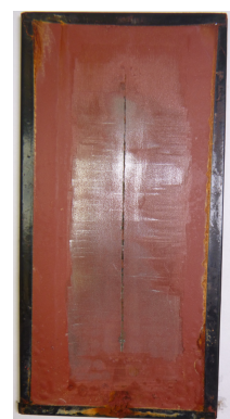
STEEL-IT® 2213 Scraped panel, 2064 h
