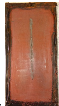
STEEL-IT 2213 + STEEL-IT 1012 (2 couches) Scraped panel, 6552 h
