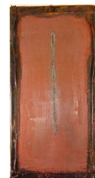
STEEL-IT 2213 + STEEL-IT 1012 (2 coats) Scraped panel, 6552 h
