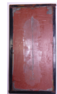
STEEL-IT® 2213 + STEEL-IT® 1002 Scraped panel, 2712 h
